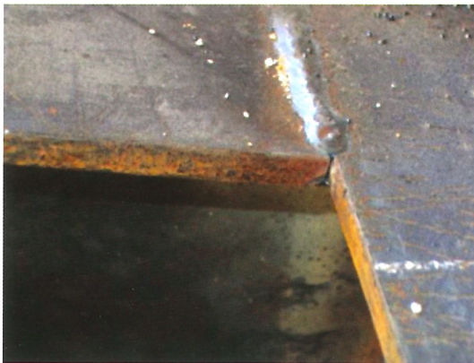
Figure 22. Penetration defects Figura 22. Defectos de penetraci3n.
