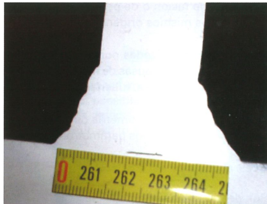
Figure 22. Penetration defects Figura 22. Defectos de penetraci3n.
